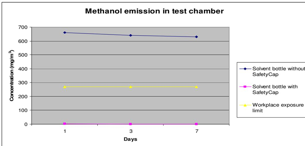
It becomes evident that with a solvent bottle without a SafetyCap in the test cabinet, despite a continual air change, a concentration of methanol of 630 — 660 mg/m<sup>3</sup> could be established, whereas with a solvent bottle with SafetyCap the results showed concentration of only 1 - 2 mg/m<sup>3</sup>.
