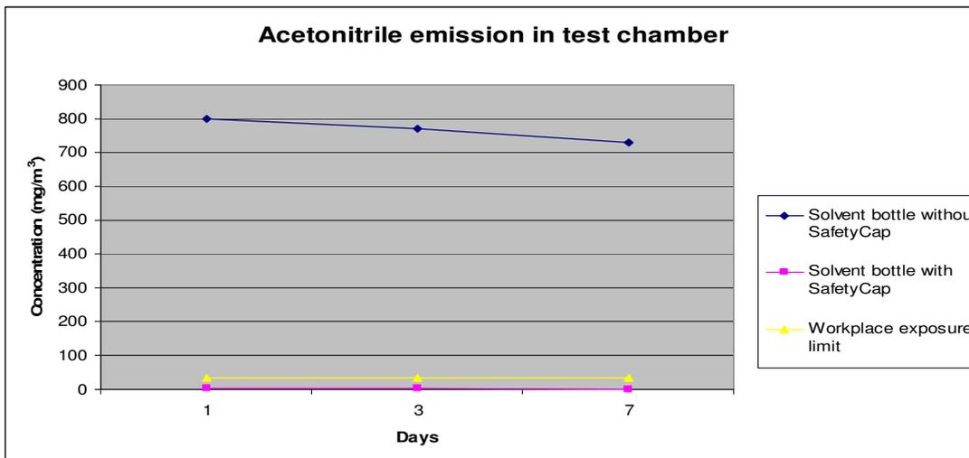
Using a SCAT SafetyWasteCap, a concentration of 1 – 5 mg/m<sup>3</sup> could be observed, while on the contrary, with the bottle without any SafetyCap, the Acetonitrile concentration, despite a continual air change, was 730 - 800 mg/m<sup>3</sup>.
