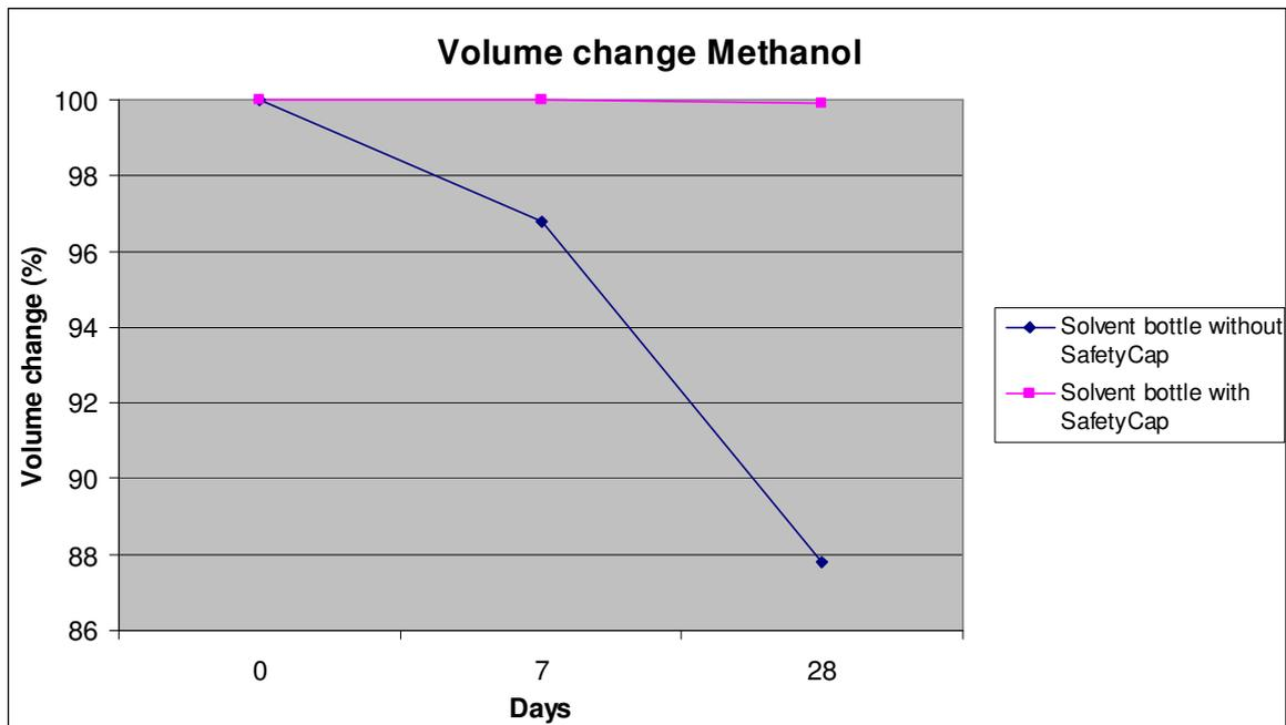
During the determination of the change in volume of methanol, it was evident that an even more significant reduction had occurred in the solvent bottle not fitted with a SCAT SafetyCap: after 28 days, only 87.8 % of the initial volume remained in the open solvent bottle, compared with 100 % of the initial volume remaining in the solvent bottle equipped with the SCAT SafetyCap.
